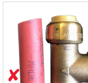
Pipe has not been cut square
